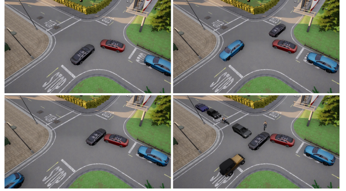
Fig. 3. Frames from replaying four representative repetitions of “Scenario 61” showing four unique behaviors. Each time, the ego vehicle (black sedan) approaches a four-way stop junction from one side and faces a red car that came on its way. Due to simulator nondeterminism, we can observe four alternative behaviors that happen next: 1) Top left : the ego vehicle ends up in a deadlock where neither car can move, triggering a ‘vehicle blocked’ infraction. 2) Top right : the ego vehicle manages to pass through the junction safely 3) Bottom left : the ego vehicle tries to pass through but collides with the red car 4) Bottom right : the ego vehicle ends up in a deadlock, causing more traffic, but tries to drive through, resulting in multiple collisions with both the red car and the motorcyclist.
