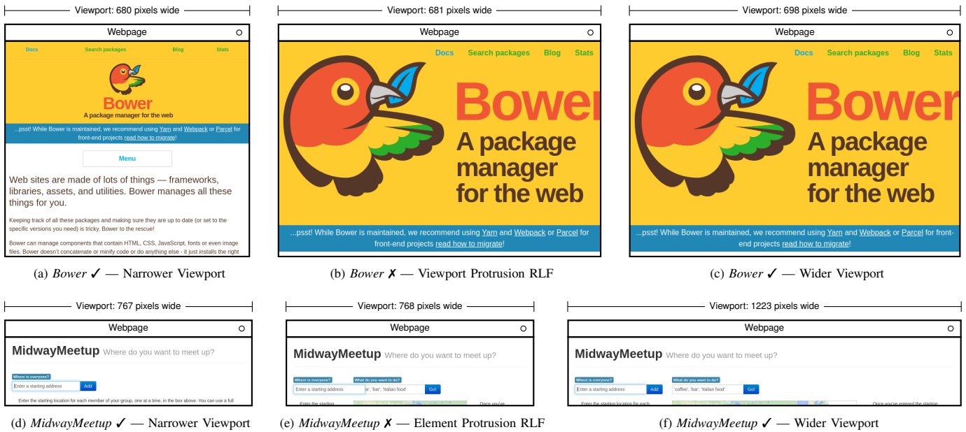
Fig. 1. Webpages with Responsive Layout Failures (RLFs), visual discrepancies that are only apparent when the page is rendered at certain viewport widths. For the Bower example, the “r” in the logo protrudes off the right edge of the viewport (part (b)). For MidwayMeetup , the first text input box protrudes into the second, and its associated button is hidden and no longer clickable (part (e)). Both pages render without issues at narrower and wider viewport widths.
