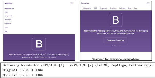
Figure 3: The original version of getbootstrap.com (top-left), the incrementally modified version (top-right), and a snippet of the report produced by REDECHECK (bottom).
