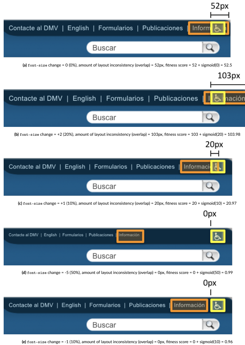
FIGURE 7 Illustration of fitness calculations for correcting the text overlap on the DMV homepage
