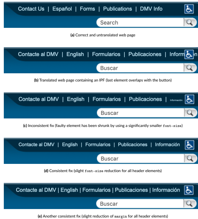
FIGURE 2 Example of an IPF on the DMV homepage when translated from English to Spanish and different ways of fixing the IPF
